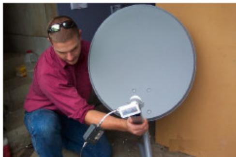
Note the SF95 meter hanging off the white coax cable to the left of the LNB.
