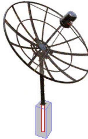
There must not be more than 1500mm between the lower edge of the dish (when the dish is at 0 deg Horizontal) and a brace. The concrete base is considered to be a brace.
